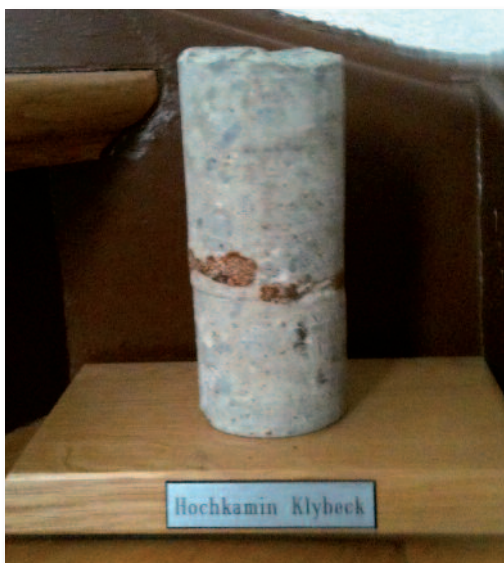
Picture of the drill core from the chimney stack; Photograph: Hans-Georg Heimann, Ownership: Renate Köhler
